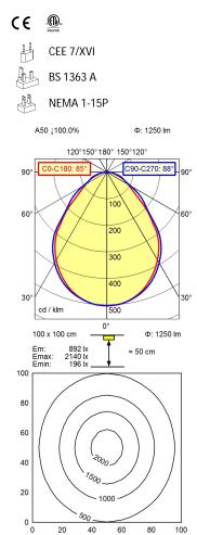
light source LED work equipment electronic plug-in ballast connected load 100-240 V, 50/60 Hz power consumption env. 16 W luminous flux approx. 1.250 lm luminous efficiency approx. 78 lm/W light type/-color cold white approx. 5.000 K colour temperatur CRI > 80 color rendering index light distribution direct direct ratio approx. 100 % beam angle 85 chromaticity tolerance LED < 5 SDCM glare control structured screen luminance (L65)  $<= 16000 \text{ cd/m}^2$
