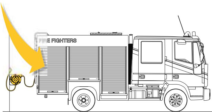
This cable is the ideal to keep emergency vehicles such as Firefighters' trucks, always plugged in to an electricity source. Thanks to this cable the vehicle can maintain its electrical parts always connected and its pressurized air tanks always charged.
